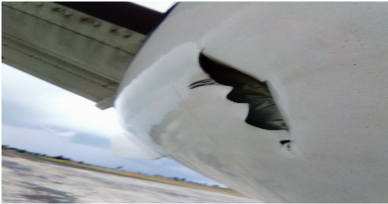
Figure 3: Picture showing damage to right side region of aircraft cargo compartment.
