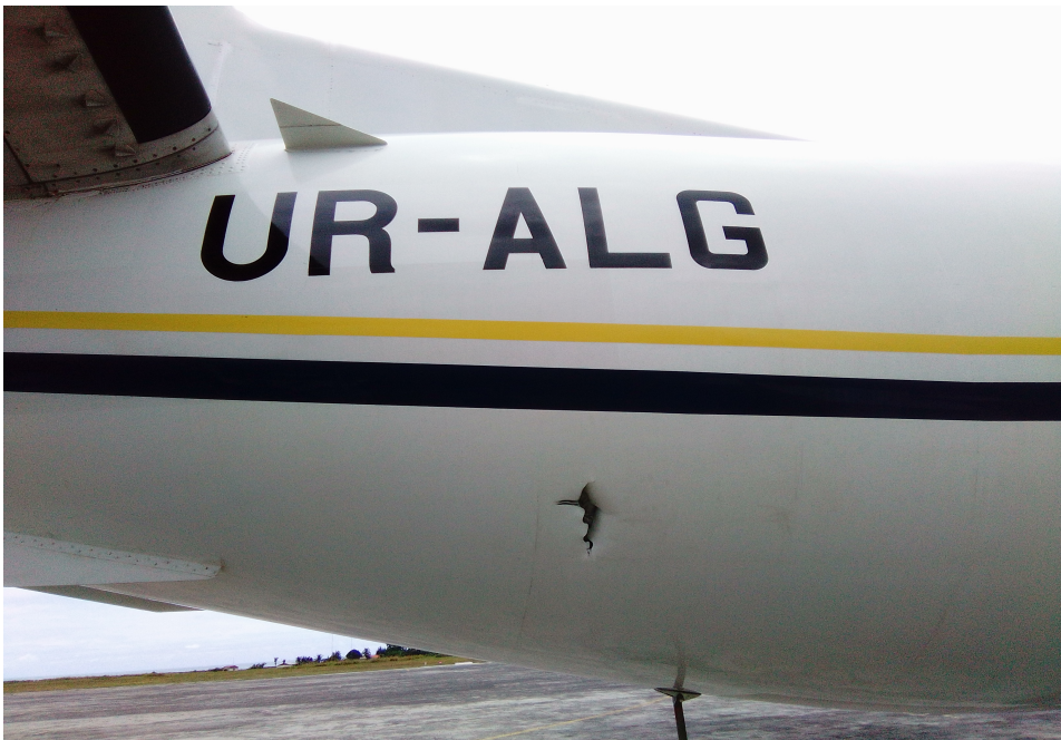
Figure 2: Picture showing damage to right side region of aircraft cargo compartment.
